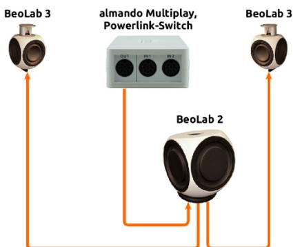
You can also connect a subwoofer. The subwoofer itself has two further Powerlink sockets to which you connect the pair of speakers.
