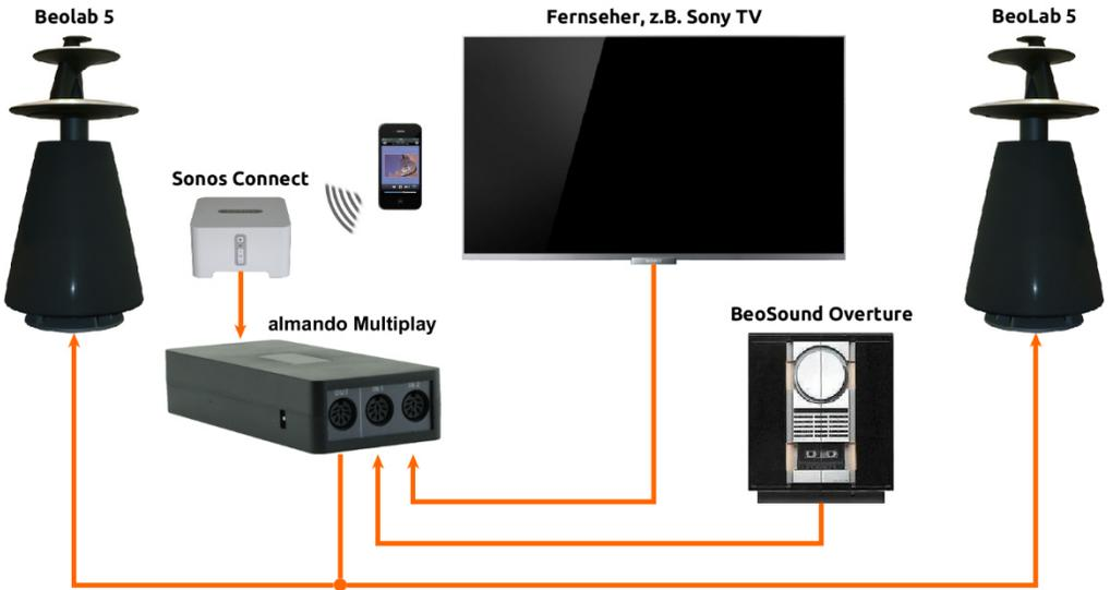
Powerlink signals from connected B&O devices are simply looped through. All other audio signals - whether digital or analog - are converted to a 100% standard B&O Powerlink signal including the trigger voltage required for the B&O loudspeakers (as well as the B&O data signal for BeoLab 5, BeoLab 4500 and BeoLab Penta if required).
