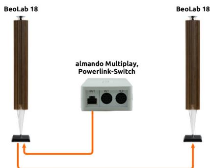
If your B&O speakers each have two Powerlink sockets, you can also loop the Powerlink cables through (daisy chain) - from one speaker to the next, like a chain of lights.
