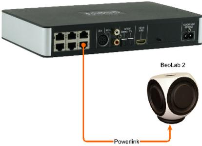
Subwoofers like a BeoLab 2 are connected to the lower right RJ45 socket.
