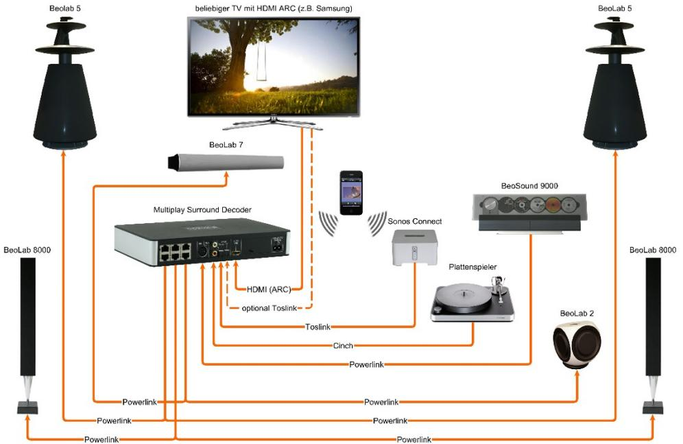
The almando Multiplay Surround Decoder can be individually configured with a smartphone app. This allows you to set all parameters such as Lipsync, Downmix, Pro Logic Mode, volume and distances of the speakers, and adjust the sound settings such as treble, bass and loudness, etc. And all of this is even partial for each input individually. This allows you to set up your surround system to your needs.
