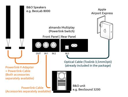
Connect an Apple Airport Express with an optical cable (optical fiber assembly) on DIGITAL INPUT (SPDIF) of the **almando Multiplay** and thereby refit your B&O unit or your B&O speakers with the Airplay function.
