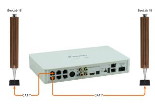
Newer B&O speakers (e.g., BeoLab 18) will be connect directly with a CAT 7 patch cable.
