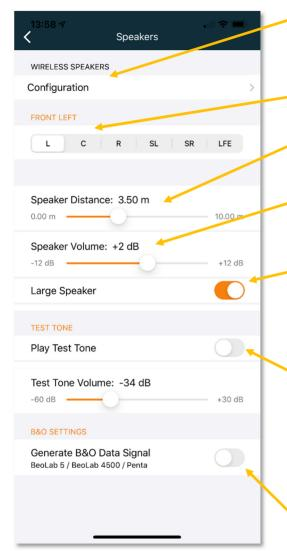
Optional: If the device has an integrated WiSA transmitter module you can open a page to connect wireless speaker (e.g. BeoLab 18).
