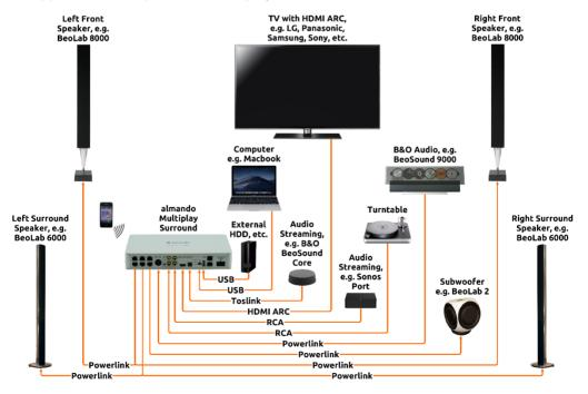
The almando Multiplay Surround can be individually configured with a smartphone app. This allows you to set all parameters such as Lipsync, Downmix, Pro Logic Mode, volume and distances of the speakers, and adjust the sound settings such as treble, bass and loudness, etc. And all of this is even partial for each input individually. This allows you to set up your surround system to your needs.
