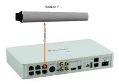
The right upper RJ45 socket is specifically designed for connecting center speakers only. The center tone is output on both Powerlink audio signals from this socket. This makes it possible to connect not just mono but also stereo speakers (as shown here with a BeoLab 7).
