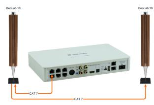
If the speakers have two Powerlink sockets, the wiring can also be made in daisy chain.
